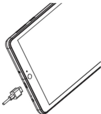
1. Insert the USB Type-C cable into the charge port as shown.
