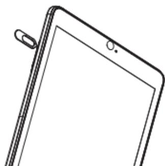
Insert the SIM pin that's provided to eject the SIM tray and then slide it out gently.
