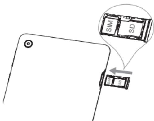
Place or remove the Nano SIM card and the microSD™ card in the correct slot as shown.
