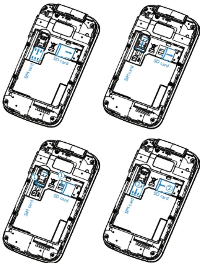
To remove the SIM card or microSD card, press down on the small plastic tab (①), then slide out the card(②). Do not use force or any sharp objects.
