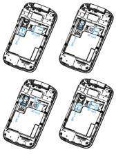
To remove the SIM card or microSD card, press down on the small plastic tab (①), then slide out the card(②). Do not use force or any sharp objects.
