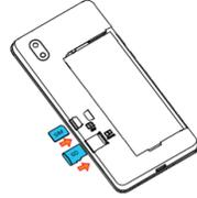
3. Ensure that nano SIM and microSD™ cards have been properly secured.
