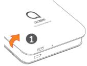
2 Installing or removing the battery.
