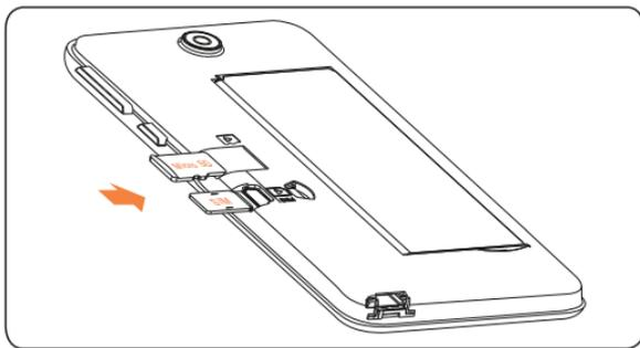
3. Ensure that SIM and microSD™ cards have been properly secured.
