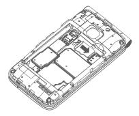
**Step 3.** To insert MicroSD card, push the MicroSD card into the card slot with the gold-colored contacts facing down.
