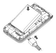
**Step 4.** Re-install the battery by aligning the gold contact points of the battery with the gold contact points of the device. It only fits one way. Press down to snap in place.
