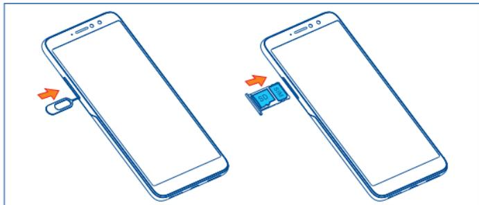
To install SIM/microSD card, place the SIM/microSD card with the chip facing downwards into the housing, and then slide it into its slot. To remove SIM/microSD card, press and slide it out.
