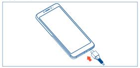
It is advised that you fully charge your battery (1). Connect the battery charger to your phone and main socket respectively, charging status is indicated by the percentage on screen while the phone is powered off. The percentage increases as the phone is charged.
