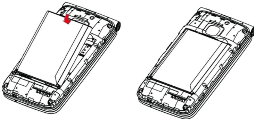
5. Attach the battery cover. Make sure all the tabs are secure and there are no gaps around the cover.
