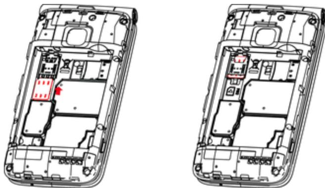
3. Insert the battery and replace the battery cover. (See [Insert the Battery](#).)
