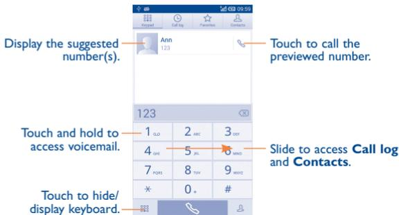
Enter the desired number from the keyboard directly or select a contact from **Contacts** or **Call log** by sliding or touching tabs, then touch to place the call.
