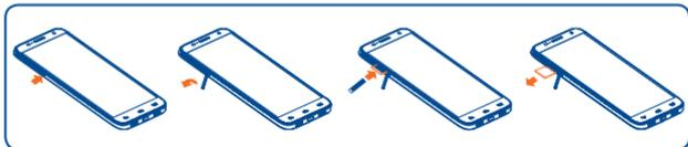
To install, place the SIM card with the chip facing downwards in to the housing, and then slide it into its slot. Make sure that it is correctly inserted. To remove the card, press and slide it out.
