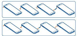
Insert the microSD card with the golden contact facing downwards into the slot.To remove the microSD card, gently press and slide it out.
