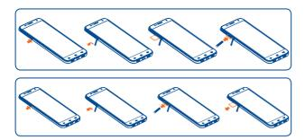
To install, place the SIM card with the chip facing downwards in to the housing, and then slide it into its slot. Make sure that it is correctly inserted. To remove the card, press and slide it out.
