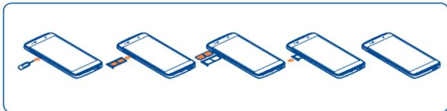
Before you install or remove the SIM card or microSD card, use the SIM card tool to press the small hole on the side of the device until the SIM/microSD tray pops out.
