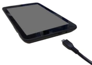
To charge tablet, connect supplied USB cable and charger to tablet micro USB port and plug into electrical outlet.
