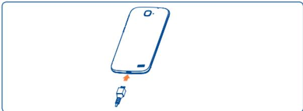
Connect the battery charger to your tablet and wall outlet.
