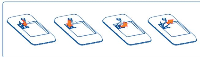
To install, open microSD card lock first, and then place the external microSD card into the slot with the gold contact facing down. To remove the external microSD card, open microSD card lock and take it out from the slot.
