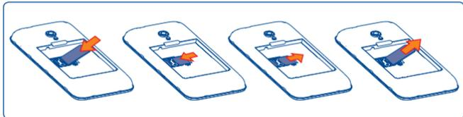
Place the SIM card with the chip facing down and slide it into its housing. Make sure that it is correctly inserted. To remove the card, press and slide it out.
