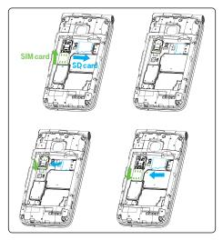
To insert Nano SIM or microSD card, push the Nano SIM or microSD card into the corresponding card slot with the gold-connectors facing down. To remove the SIM or microSD card, push down on the plastic clip located under card and push the SIM or pull microSD card out.
