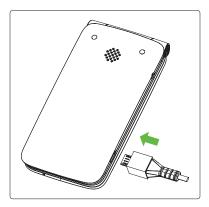
Insert the smaller end of the charger into the device charging port, and plug the charger into an electrical outlet.
